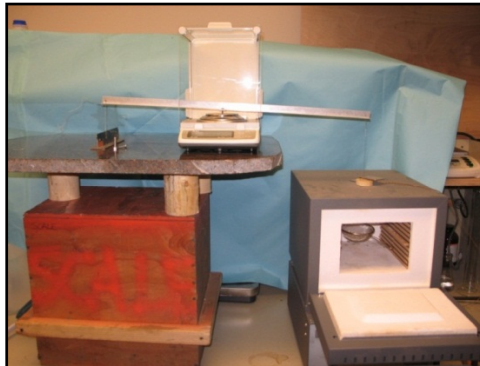
Figure 2. Natural air convection real-time mass measurement apparatus.
