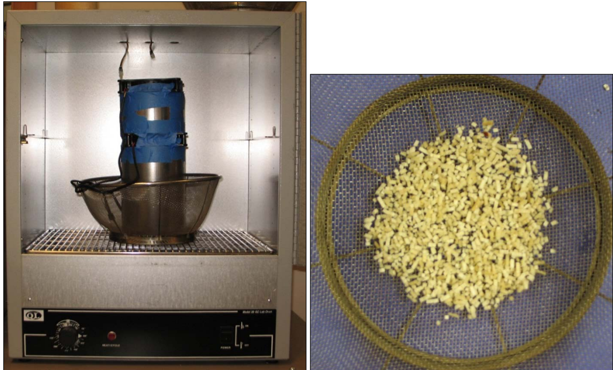
Figure 4. Left) Forced air drying apparatus. Right) Dispersion of 10g (wet) 2mm Crumbles particles for forced air drying experiment, ~ 3.3g of OD wood.
