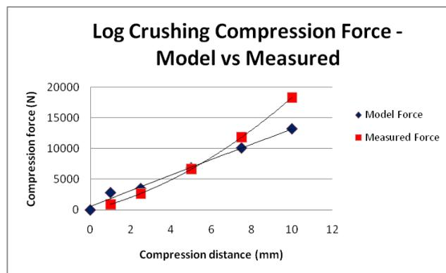
**Figure 9.** Graph of the calculated compression force (N) versus measured force for a 300 mm diameter roller acting on a 100 mm diameter round log.
