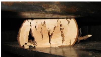
**Figure 5.** Flat plate compression of round log section vividly demonstrates the progressive failure and wedge formation due to internal Poisson's forces.
