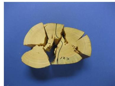
**Figure 3a, b.** The Douglas fir and lodgepole pine rounds failed into similar triangular pieces. The black lines were drawn vertical along the centerline prior to compression.
