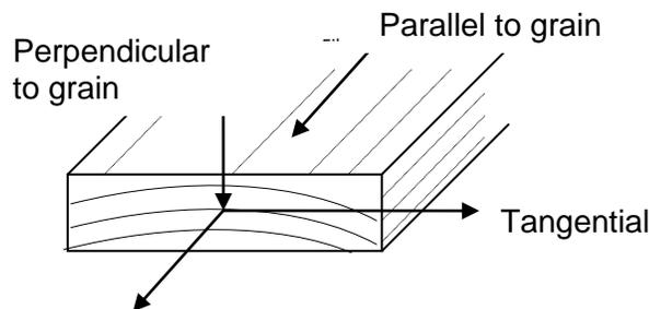
**Figure 2.** Three principal axes of wood with respect to grain direction and growth rings (Forest Products Laboratory, 1999)
