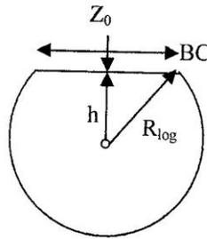
**Figure 7.** Schematic showing parameters for calculation of chord length (BC) for roundwood under compression from above.
