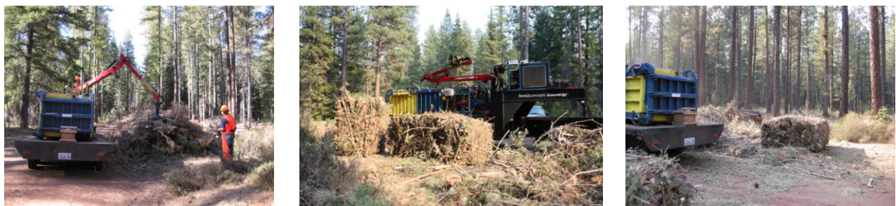
Figure 9. Baling tops and limbs from roadside thinning on the Deschutes National Forest.
