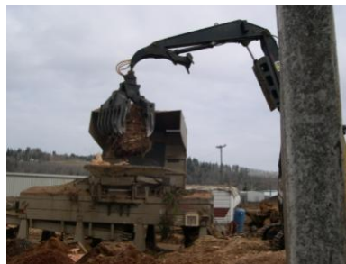
Figure 7. Baled City of Auburn woody biomass was shipped in standard trailer to Grays Harbor Paper where it was ground into hog fuel for their cogeneration plant.
