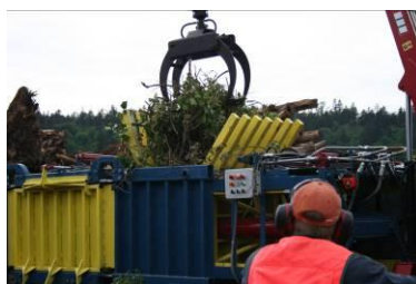
Figure 5. Field trial of prototype biomass baler at BRC Inc. yard waste facility in Auburn, WA.
