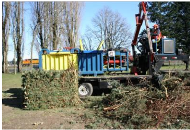
Figure 6. Field trial with City of Auburn, Washington to bale brush from parks and road maintenance operations.
