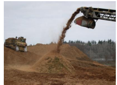
Figure 7. Baled City of Auburn woody biomass was shipped in standard trailer to Grays Harbor Paper where it was ground into hog fuel for their cogeneration plant.
