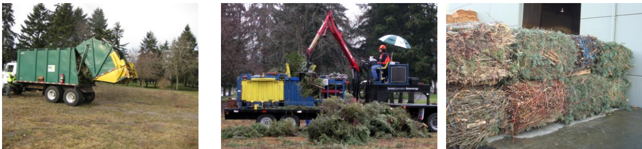
Figure 11. Route truck unloading whole Christmas trees and baling into high density bales for shipping to biopower customer. Photo of completed bales includes some bales from other hardwood prunings as well as the Christmas tree bales.
