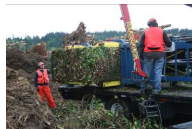
Figure 5. Field trial of prototype biomass baler at BRC Inc. yard waste facility in Auburn, WA.
