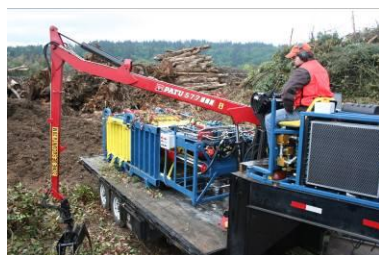
Figure 5. Field trial of prototype biomass baler at BRC Inc. yard waste facility in Auburn, WA.
