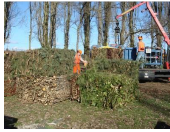
Figure 6. Field trial with City of Auburn, Washington to bale brush from parks and road maintenance operations.
