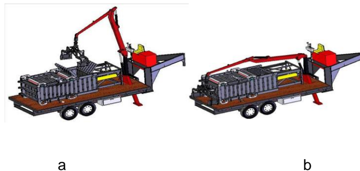
Figure 3. Computer model of self-loader trailer with prototype baler and specially designed grapple as engineered in November 2007.
