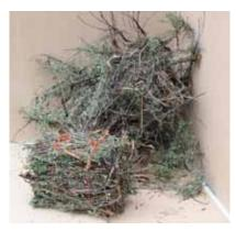
**Figure 4.** Seven kilogram (15 lb) bale of bitterbrush in the front and similar mass of bulk bitterbrush in the back. Volume reduction is approximately 5:1.
