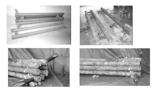
**Figure 1 a,b,c,d.** A small model was used to prove the concept of building large diameter structures from pairs of small diameter logs. A full-scale prototype was fabricated from forest residuals using a mix of western red cedar, hemlock, alder and Douglas fir logs.
