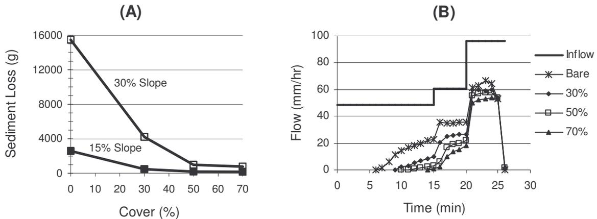
**Figure 2:** Sediment loss (A) and runoff hydrograph (B) for varying cover amounts of wood strands.
