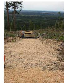
Plots were randomly assigned to treatments, with the upper plot being wood-strands at 50% cover, then bare soil control, wheat straw at 90% cover and finally wood-strands at 70% cover at the base of the slope. Hand crews applied all mulch treatments.
