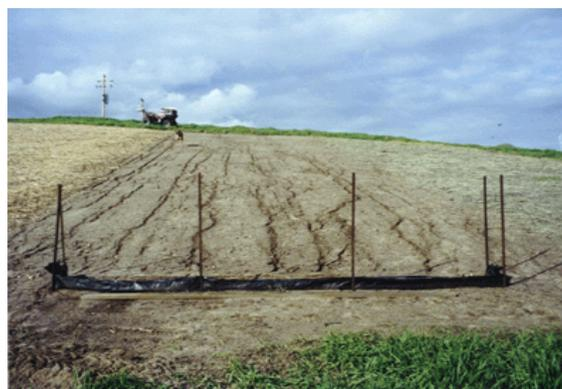
**Figure 7:** Ernst site on January 3, 2005 with wood-strand plot on the left, bare soil in the center, and barley straw plot on the right. As of this date, neither of the treated plots showed any signs of rill erosion while the bare soil plot is heavily eroded.
