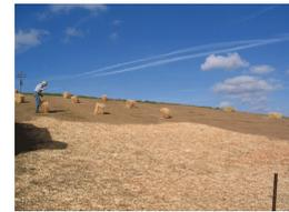
The test plots were sprayed with a broad-spectrum herbicide (Roundup) one week after the plots were installed, and monthly since that time. Herbicide applications ensure that the results are not confounded by the development of vegetative cover and root mass.
