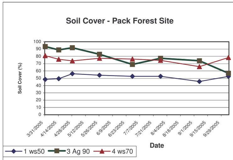
**Figure 10.** Soil cover for erosion control treatments on the Pack Forest field trial site.
