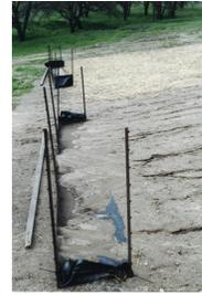
All materials were hand-spread to a target ground cover. The barley straw mulch was applied to a target cover of 90%, and the WoodStraw™ mulch was applied to a target cover of 70%. These application rates are consistent with generally accepted practice for straw mulch, and the laboratory-based optimum for WoodStraw™ mulch on highly erosive granitic soils.
