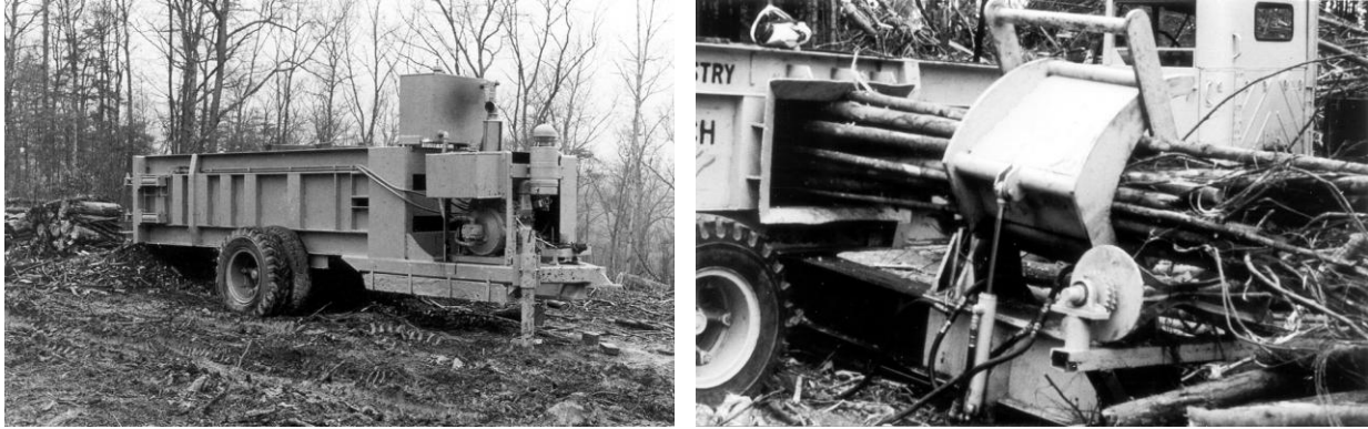
Figure 2a, 2b. VIP prototype baler overview and baler infeed gripper pushing set of smallwood stems into baler. Baler shears excess material as the plunger strokes. (P. Schiess photos)
